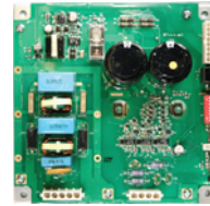
EPC Control Board
